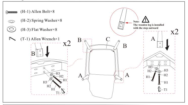
Insert the Front Legs (Ax2) and Back Legs (Bx2) into the corresponding four slots on the bottom of Seat (C) as shown. Attach the legs with Allen Bolt (H1x8), Spring Washer (H2x8), Flat washer (H3x8) using the provided Allen key(T-1), stacking the hardware in the order as shown.**DO NOT yet fully tighten.**
